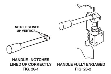
18. Raise the PLATFORM as follows. Insert MANUAL BACKUP HANDLE in Manual Pump actuator. Pump the handle up and down (FIG. 26-2) until PLATFORM is raised up even with the vehicle floor (FIG. 26-4) and Inboard Rollstop lowers to rest on Threshhold Plate.
